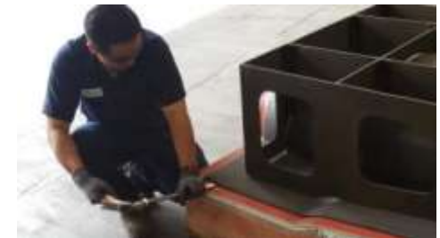
Demolding with metal wedges:
