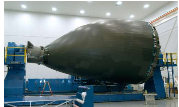
CFRP BMI was used for this tool due to weight and rotational force considerations on AFP machine.
