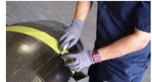
Demolding with metal wedges:
