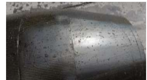
Composite tool exposed to moisture:
