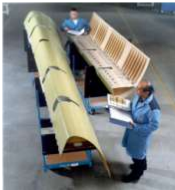
Fig. A380 thermoplastic J-nose (Fokker)
