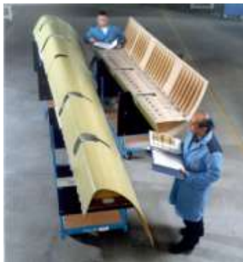
Fig. A380 thermoplastic J-nose (Fokker)
