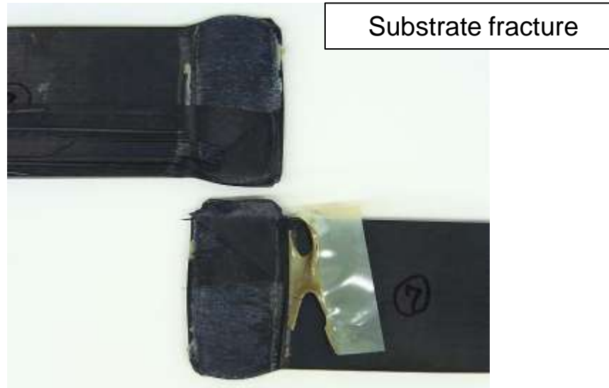
Fig. Fracture surface after single lap shear test
